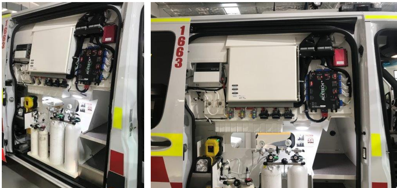
Figure 8 Current configuration of the Oxy bay
