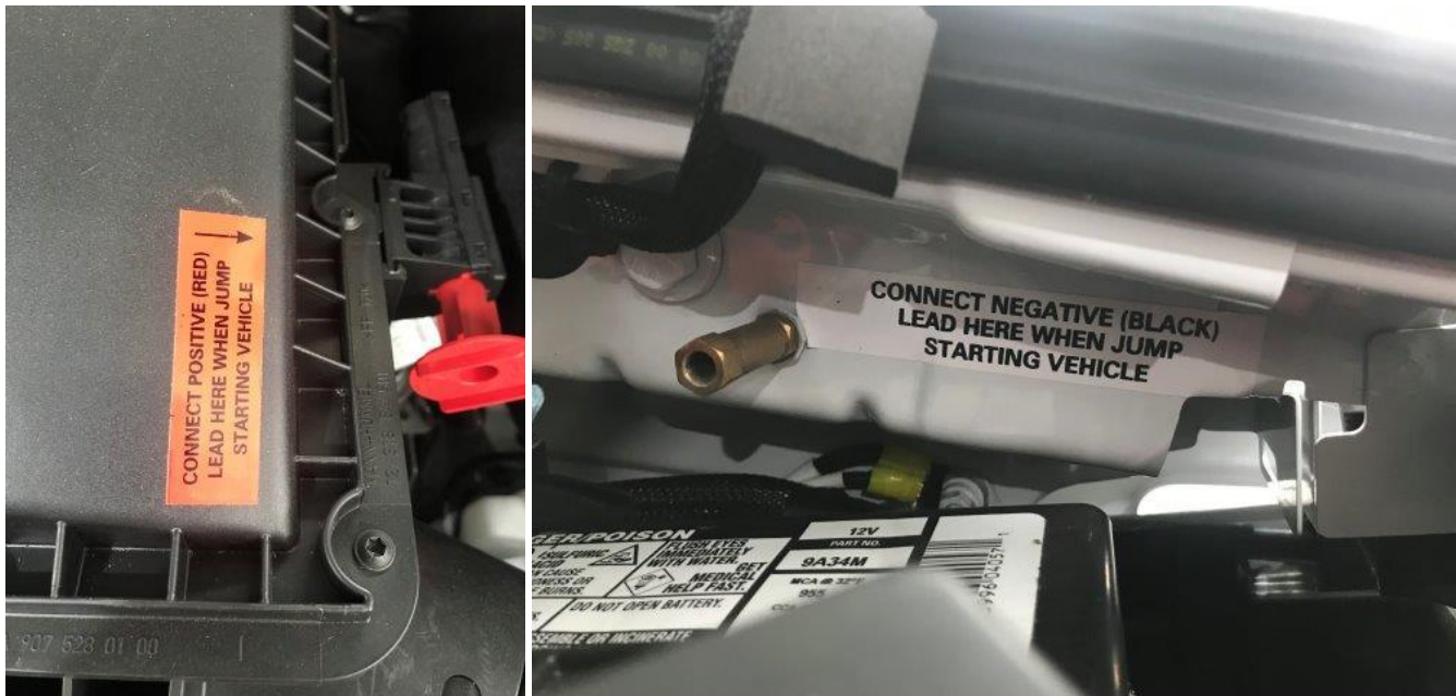
Figure 16 Jump start stickers for auxiliary battery
