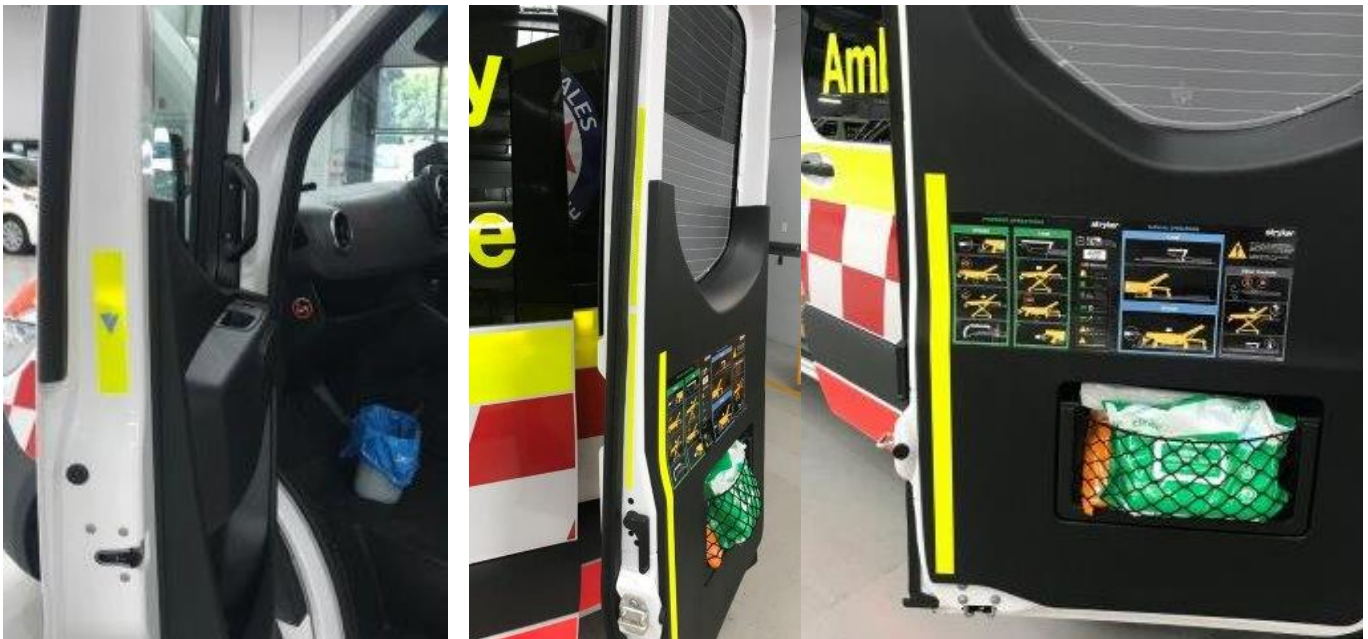
Figure 1 Yellow markings on open doors
