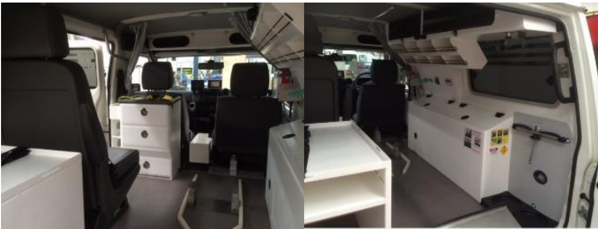
Figure 21 Layout of Amb4 Patient Compartment
